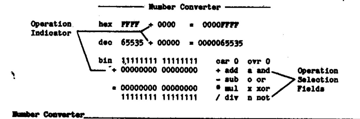
The Explorer's Number Converter will convert Hexadecimal, Decimal and Binary numbers and perform the mathematical and relational operations of Add, Subtract, Multiply, Divide, AMD, OR, XOR and NOT. The valid range for the different number bases is >0000 thru >FFFF, 0 thru 65535 and 000000000000000 thru 111111111111111111. This Number Converter operates dynamically in that ALL of the Number Converter fields are automatically updated as you type in EACH character, so type slow.
