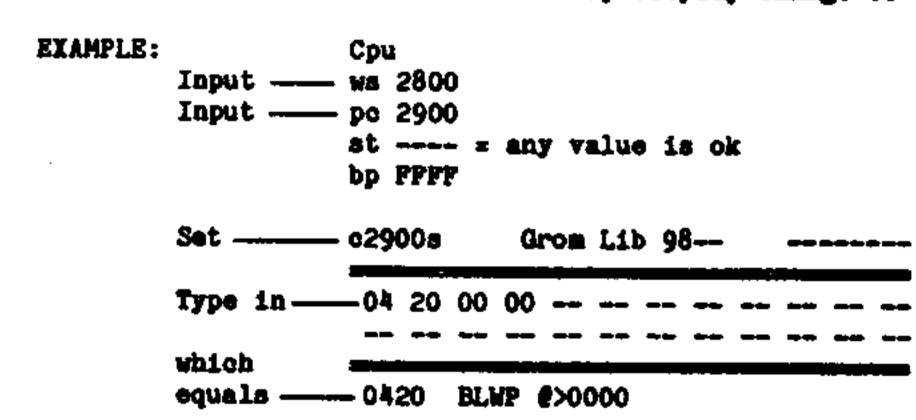
By inputting the values indicated and typing in >04 20 00 00 into the Memory Window you will set the next instruction to do a Branch and Load Workspace Pointer @>0000. This will begin execution of the Power Up routine when you press CTRL 1 or CTRL 2. Go shead and press CTRL 1 and note R13, R14 and R15 of the new Workspace.
